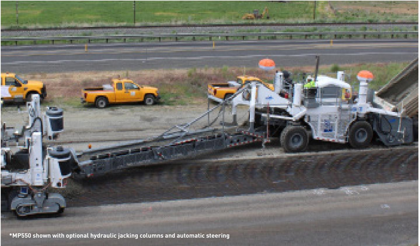
\*MP550 shown with optional hydraulic jacking columns and automatic steering
